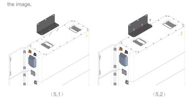
**Step 6**Drill three holes of in the wall and insert three screw plugs.Insert three screws to secure the L-shape wall hanging bracket to the wall.
