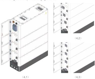
**Step 5**Attached the L-shape wall hanging bracket onto the high voltage box as shown in
