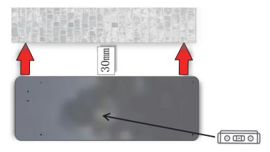
Note: Levelness of the base is less than 2mm.
